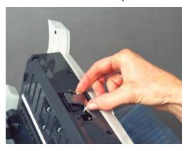
2. Wipe the feed module from top to bottom with a roller cleaning pad.
